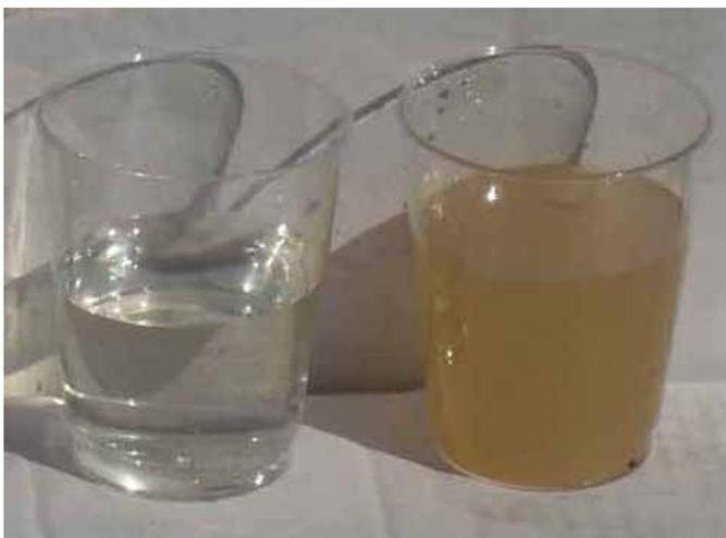
To determine the most appropriate polymers to use, the site soil was tested. This testing helped determine the reaction time required to cause sediment to drop out of the turbid storm water. Then, after assessing the expected flow rate, the treatment channel could be designed and sized accurately.
